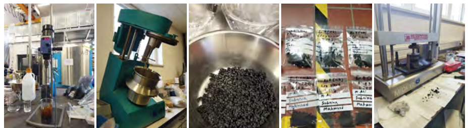
Fig. 4: Process sequence of granulation and testing in high intensity mixer
