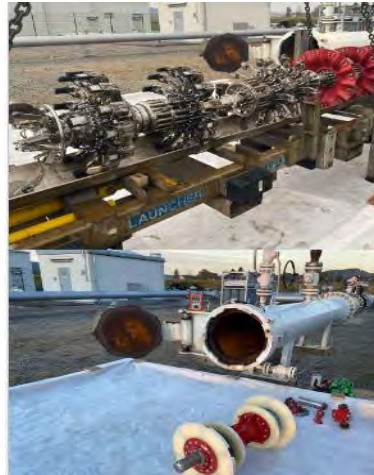
Pigging tool for pipeline inspections
