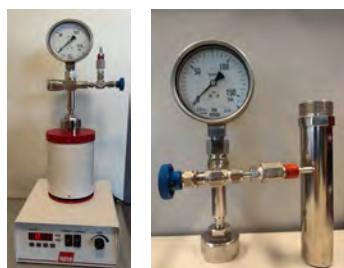
Instrumental set-up for oxidation of carbon in autoclaves with jacket (left) and without jacket (right)
